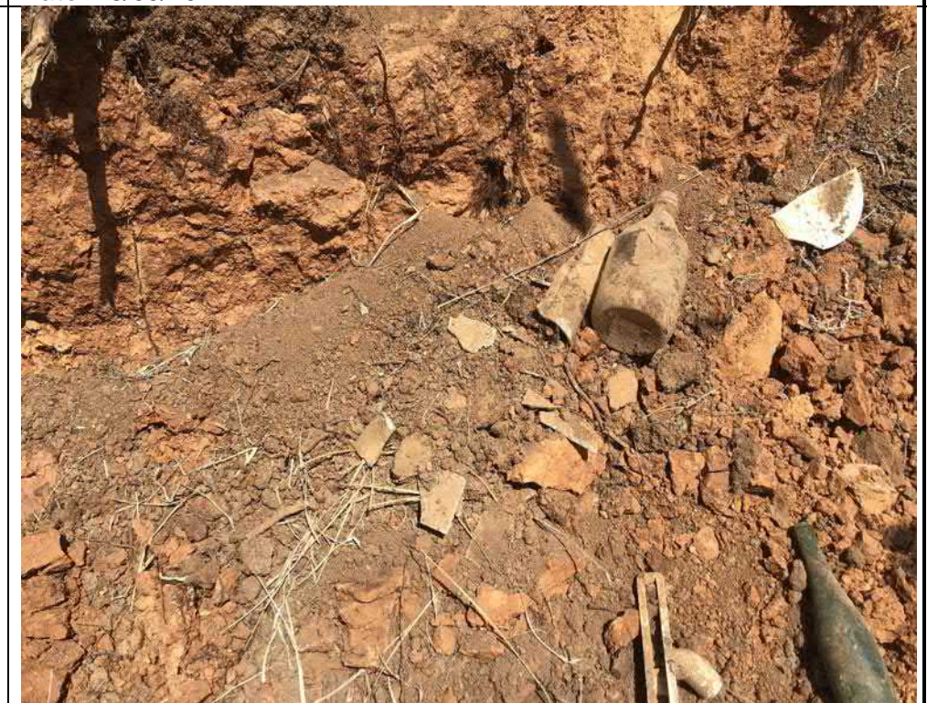
Photograph 18 – Example of anthropogenic material including ACM
