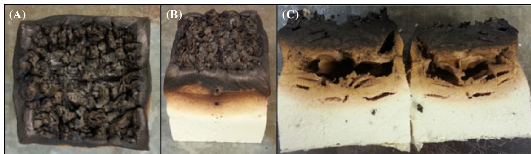
FIGURE 10 PIRa sample residue at 25 kW/m 2 without protective layer up to 22.5 minutes A, top view, B, lateral view, and C, lateral view from section. PIR, polyisocyanurate [Colour figure can be viewed at wileyonlinelibrary.com]
