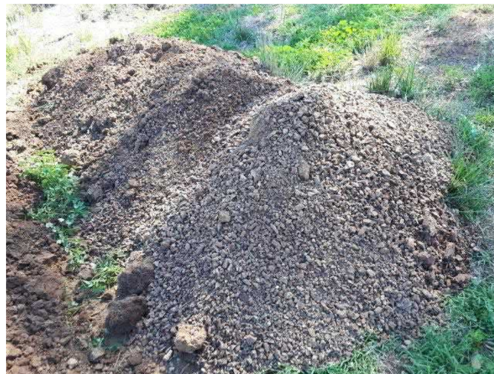
Photograph 11 – Excavated soil from test-pit
