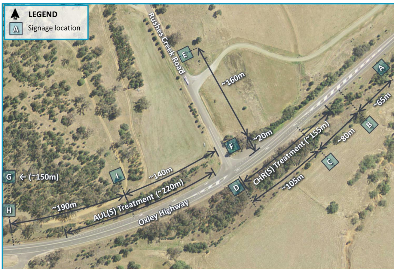
Figure 1 Oxley Highway/Rushes Creek Road - Existing Intersection Form and Signage
