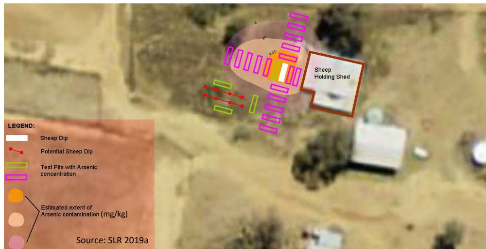
Figure 11 Arsenic Contamination Delineation 0.6-0.8 m Deep
