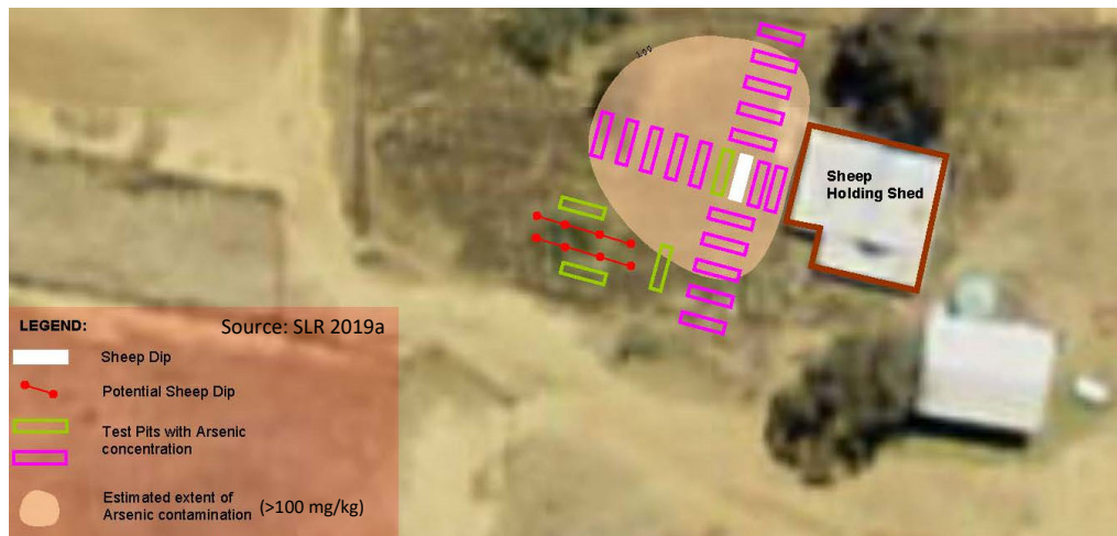
Figure 13 Estimated Arsenic Contamination (>100 mg/kg) Extent 0.1-0.2 m Deep
