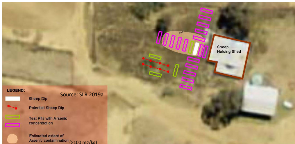
Figure 14 Estimated Arsenic Contamination (>100 mg/kg) Extent 0.6-0.8 m Deep
