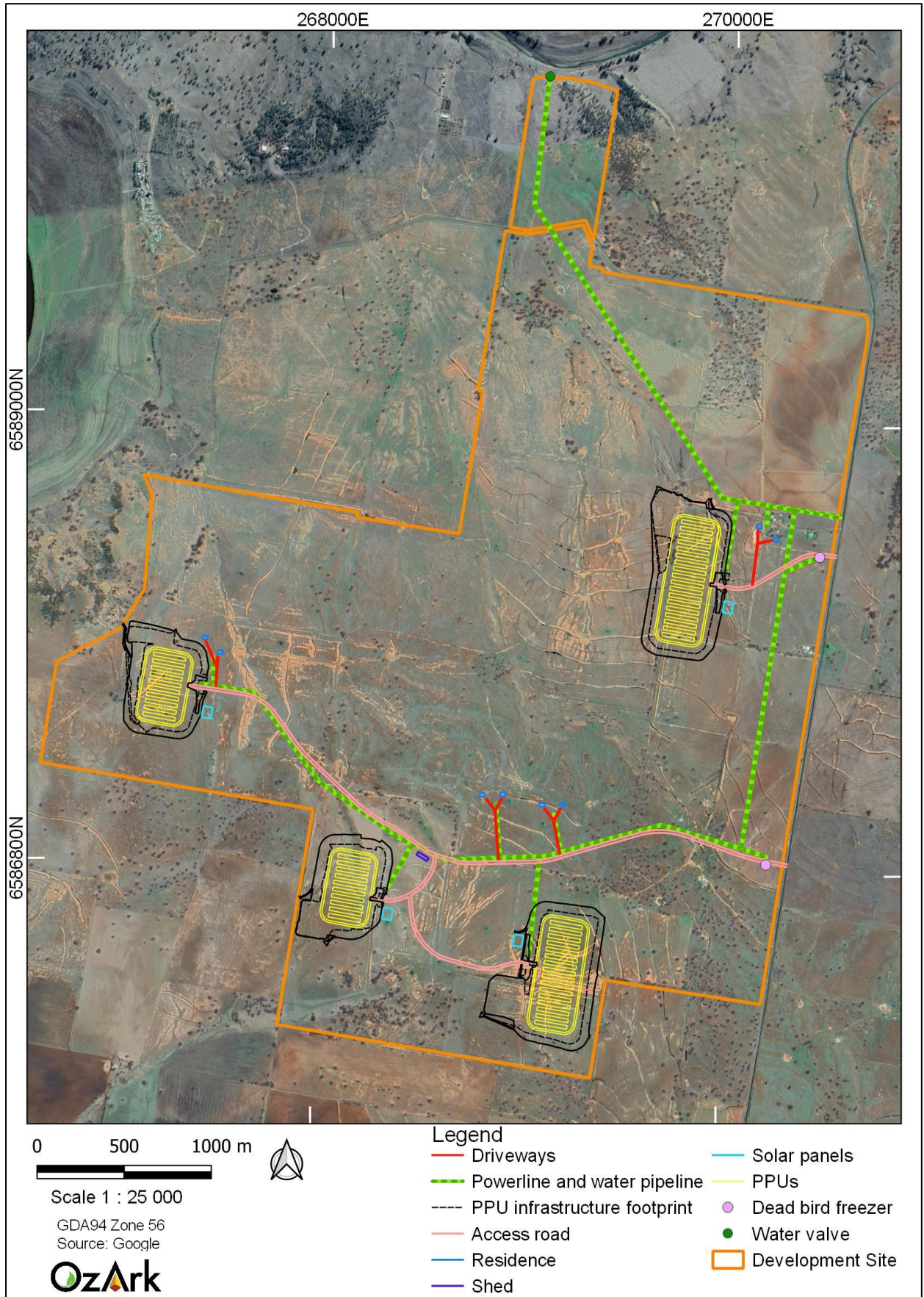
Figure 1-2: The Development Site and infrastructure layout.
