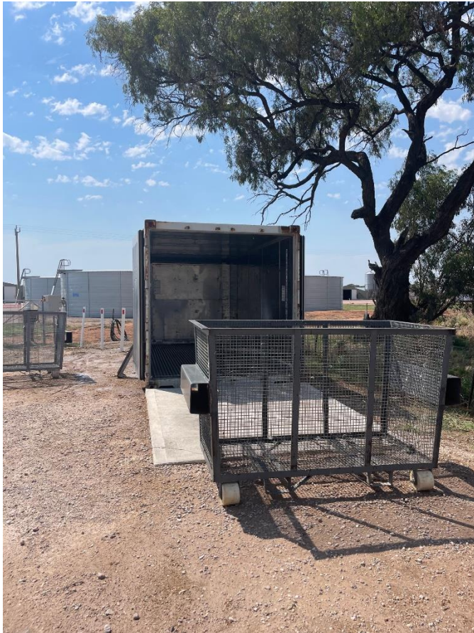
Photo 9 Mortalities to be stored in chillers prior to pick-up for disposal at the rendering plant. The Development has changed their approach in the mortalities storage, as the site changed from specific storage containers which required the specific chiller set-up established. However, ProTen changed to chillers for each PPU in this audit period and they have found this to be more suitable in terms of biosecurity.
