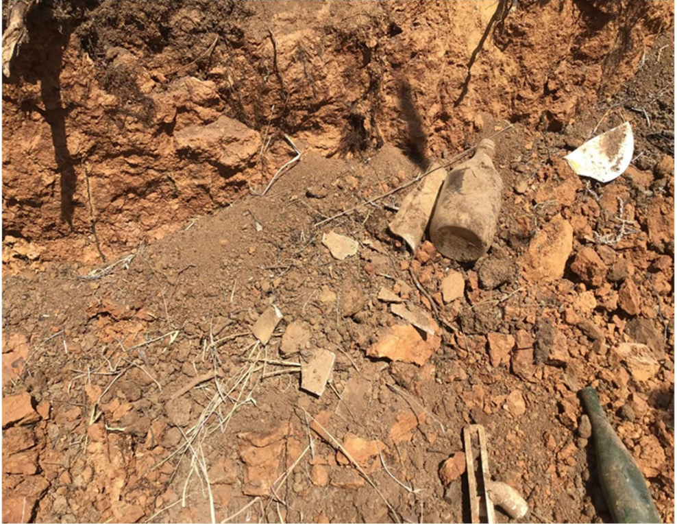
Photograph 18 – Example of anthropogenic material including ACM
